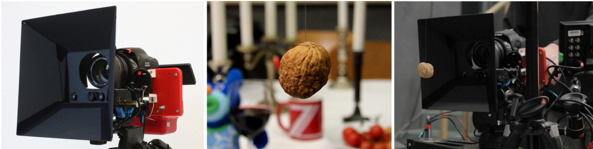
Figure 1: Left: A DSLR video rig with an integrated Kinect. The Kinect is used as an external rangefinder and for 6DOF tracking. Center: Continuous focus on a small walnut in a dolly shot (detail from a video). Right: The camera moving very close to the nut and maintaining focus automatically.
